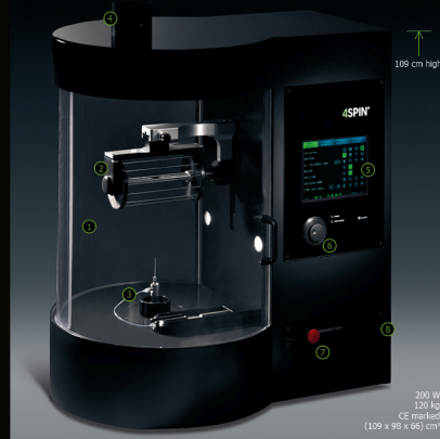
Legend: 1) Deposition chamber, 2) Collector, 3) Emitter with integrated dosing system, 4) Exhaust pipe, 5) 10.4" touch screen, 6) Multifunctional knob, 7) Central stop, 8) Terminals.
